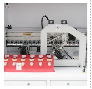
Cabinet door edge banding, edge banding corner rounding chamfering process integrally formed. Two high-speed motors are chamfered, and each motor repairs two corners on the upper or lower side, which takes up less space on the fuselage, and is relatively simple to debug, economical and practical. The technical precipitation time is long, and the functional structure is mature and stable.
