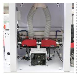
Double diamond cutter head structure, two reverse cutting cutter heads, no edge chipping during milling, smooth and burr-free milling surface, simple and convenient adjustment, standard 55 cutter head, other requirements can be customized. After pre-milling, the surface of the board is blown to dust.
