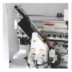
With Endcutting function, two Endcutting motor share one guide rail. It takes a long time for the technology to settle down, the functional structure is mature and stable, the space occupied by the fuselage is short, and the debugging is convenient and simple. Equipped with an automatic oiler, it can be automatically oiled and maintained to the rails at regular intervals.
