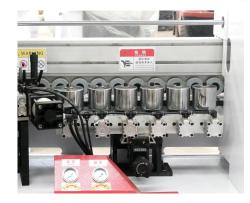
3-6 wheels for press-fit edge banding can be customized. The first pressing wheel, vertical surface pressing, active wheel, and feeding shaft synchronous rotation, to prevent the sealing tape front and back misalignment. The second and fourth press wheels are tilted down on the press surface to press the edge of the sealing belt; the third and fifth press wheels are tilted on the press surface to press the edge of the sealing belt. The last straight wheel is pressed on the vertical side.
