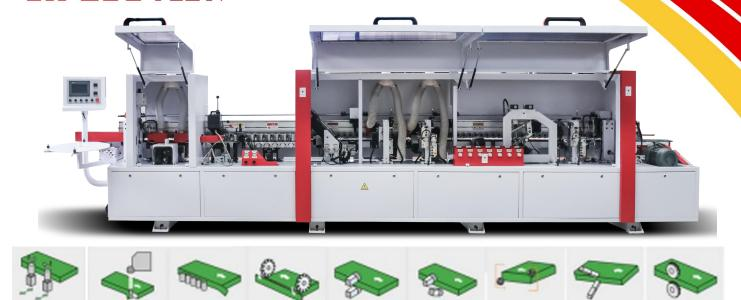
$Pre-milling \rightarrow Adhesive \ edge \ banding \rightarrow Endcutting \rightarrow Rough \ trimming \rightarrow Fine \ trimming \rightarrow Corner \ Rounding \rightarrow Scraping \rightarrow Polishing$
