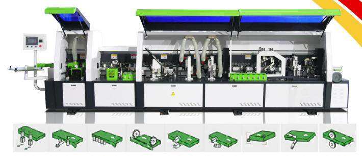
$Pre-milling \rightarrow Adhesive \ edge \ banding \rightarrow Endcutting \rightarrow Rough \ trimming \rightarrow Fine \ trimming \rightarrow Corner \ Rounding \rightarrow Scraping \rightarrow Polishing$
